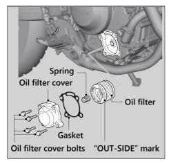
Install a new oil filter with the "OUT-SIDE" mark facing out. **8.** Install the spring into the oil filter cover, and then install a new gasket and oil filter cover by tightening the oil filter cover bolts.
