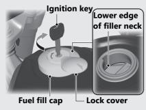
Do not fill with fuel above the lower edge of the filler neck
