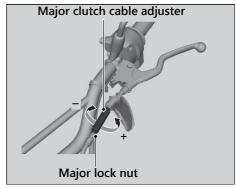
If proper adjustment cannot be obtained or the clutch does not work correctly, see your dealer
