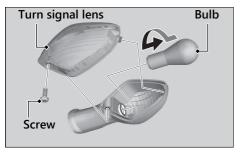
**4.** Install a new bulb and parts in the reverse order of removal.
