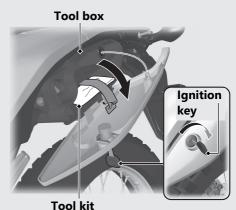
► Insert the ignition key and turn it clockwise to open the tool box.
